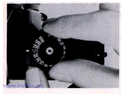
1. Press the Shutter Speed Dial Release Button. and set the Shutter Speed Dial to the desired shutter speed.
